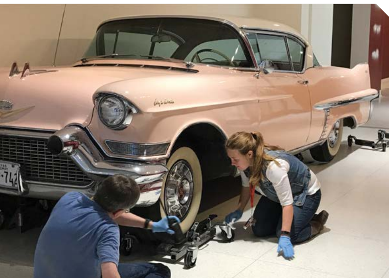
The first step to moving the Museum's '57 Caddy back into storage involved jacking the 4,800-pound automobile up to slide dollies under each wheel so it could roll down the hallway. The Cadillac is arguably the heaviest object in the Museum's collections.
