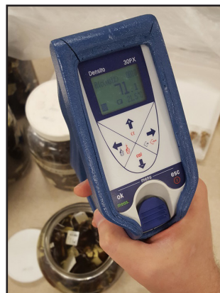
Using a density meter to determine the ethanol concentration of fluid.
