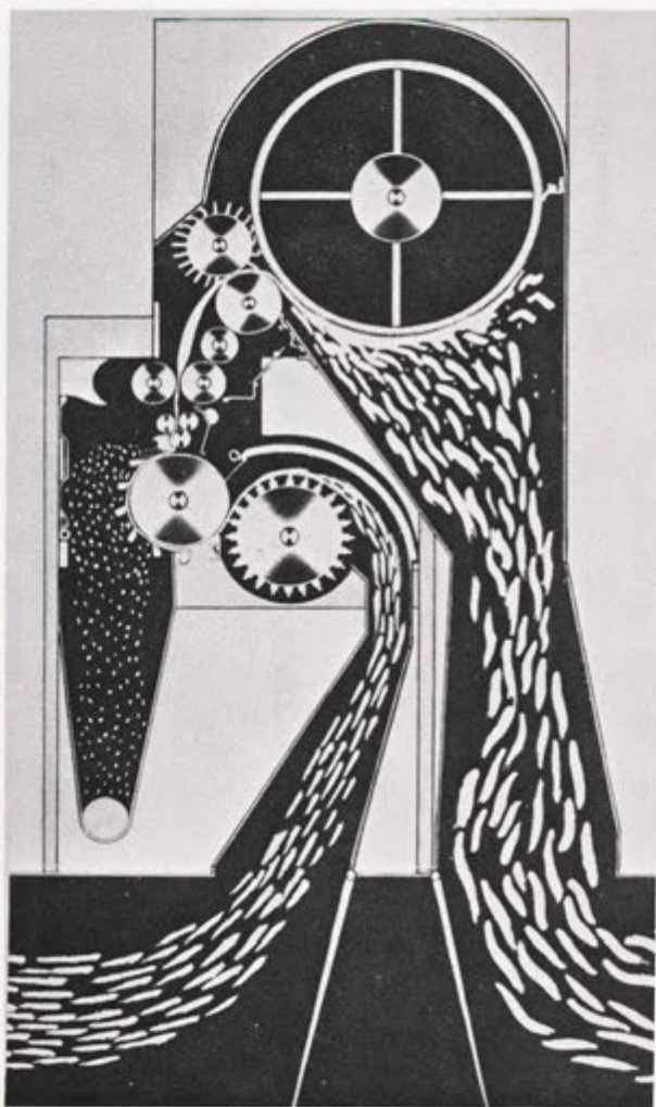
FIGURE 3-44.—Bulk saw lint cleaner (Bush-Hog/Continental Gin Cleanmaster lint cleaner).
