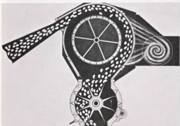
FIGURE 4-5.—Separator with revolving screen drum (Bush-Hog/Continental Gin).
