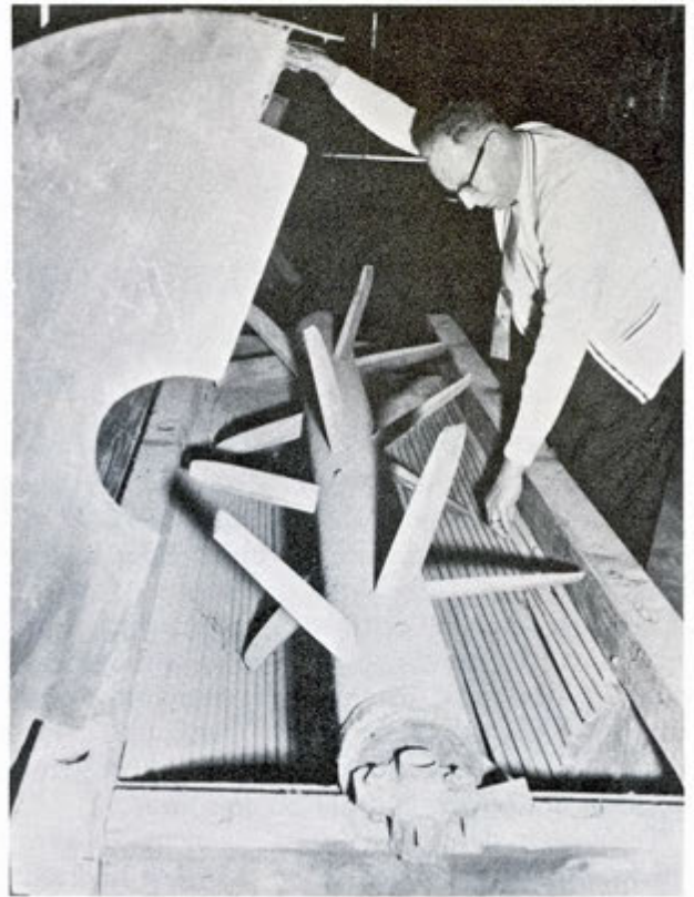
FIGURE 1-3.—Wooden seed-cotton cleaner built by a slave for the Blakely Plantation Gin north of Vicksburg, Miss.
