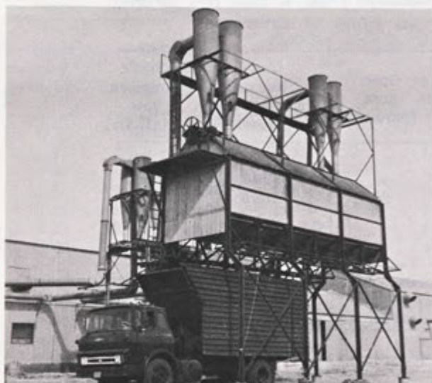
FIGURE 4-35.—Typical bur hopper and spreader truck used extensively in stripper-harvesting areas.
