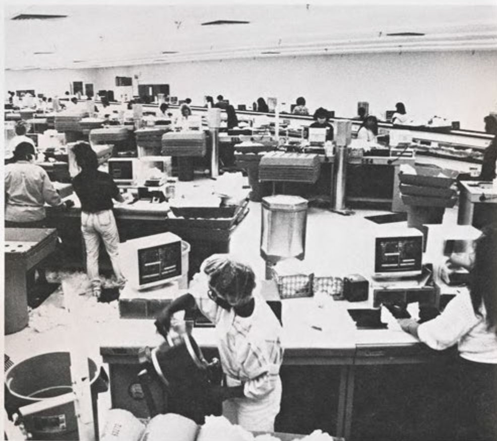
Utilizing the latest technology and equipment, samples are classed on an assembly line arrangement with fiber measurement results electronically transmitted to the classing facility's computerized data base.
