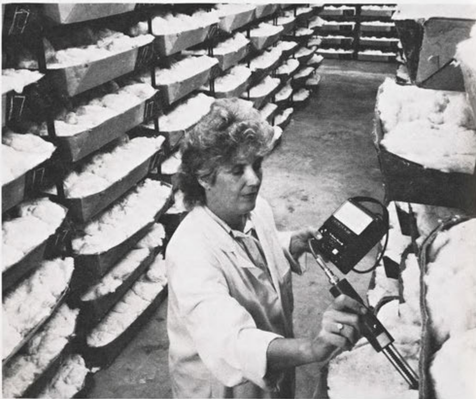
Upon arrival at the USDA classing facility, samples are conditioned to standardize moisture content before the classing process begins.
