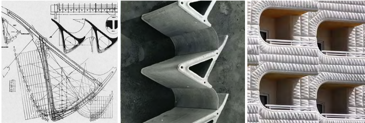
Miguel Fisac's Component Drawing and Prototype; Miguel Fisac's Hotel Tres Islas Facade
