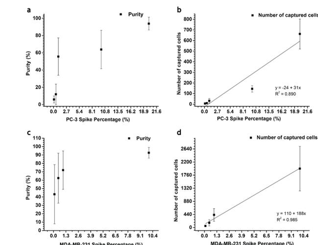
Graphs a-d show the purity and number of cells captured from the concentration studies for PC-3 and MDA-MB-231. LOD was 1 cell/ $\mu$ L concentration. At a 0.1% spike to lysed blood, PC-3 cells were captured at 34  $\pm$ 5% purity and MDA-MB-231 cells at 43  $\pm$ 35% purity.
