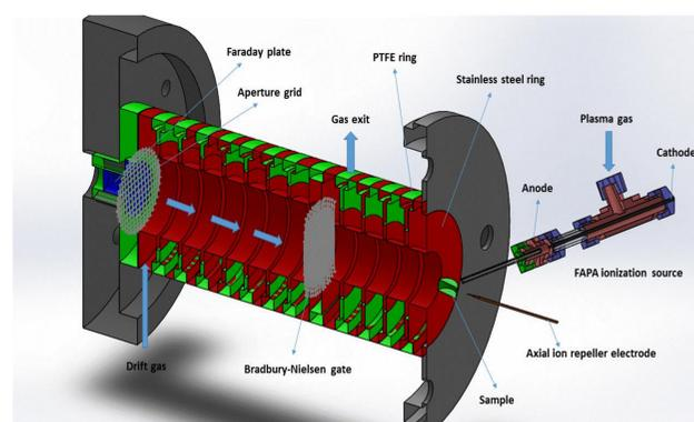
Figure 3. Drift Tube Ion Mobility Spectrometer schematic diagram cross section.
