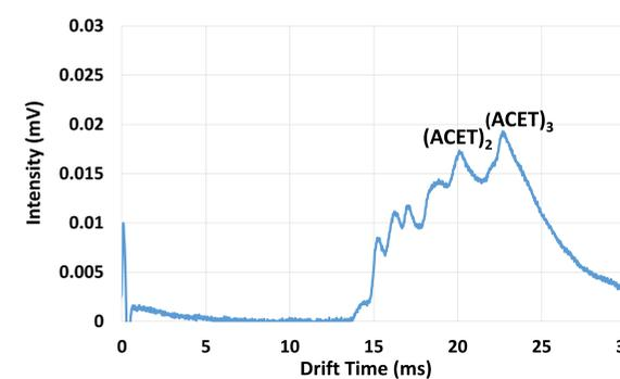
Figure 8. Ion mobility spectrum of dimer and trimer of acetaminophen at 20.1 and 22.5ms, respectively ( $\text{ACET}_2$  and  $\text{ACET}_3$ ).
