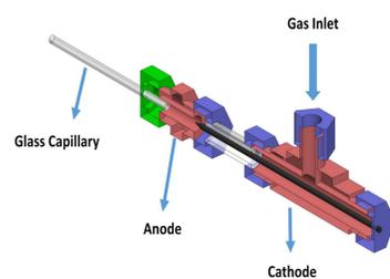
Figure 2. Section view of FAPA.
