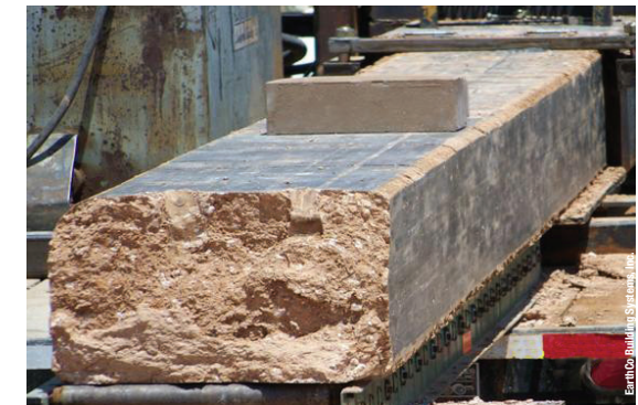
This EarthCo Megablock™ measures 18 inches wide by 12 inches tall, is over 14 feet long, and weighs more than 1 ton.
