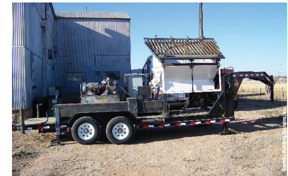
The EarthCo Megablock™ machine is able to convert soils into giant modular building blocks called EarthCo Megablocks™.
