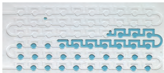
A one microliter water plug containing blue food color dye entering into the network, fragments at each parking spot leaving a remnant of the plug. This approach enables rapid immobilization of large number of parked drops consuming only nanoliter reagent volumes for each drug reaction.
