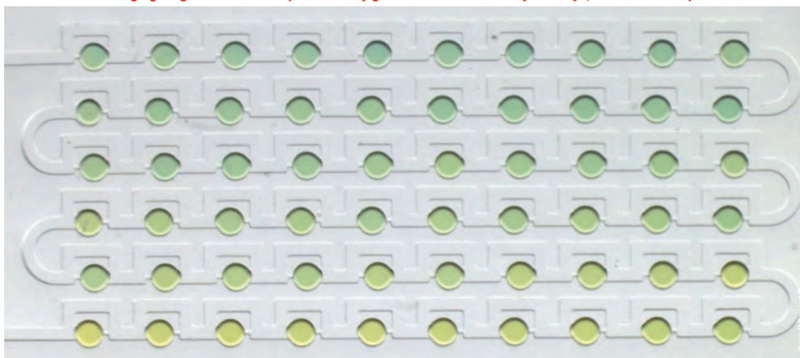
This approach allows generation of reagent variation from drop to drop in the array, offering a simple and inexpensive dilution method for rapid drug screening.
