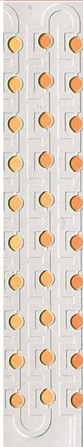
When a yellow-colored water plug is introduced in the microfluidic parking network, it merges with each of blue parked drop, exchanging reagent. The first drop in the array gets the most amount of yellow dye, and the last drop the least amount.
