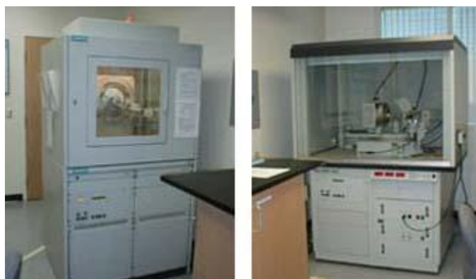
Figure 1: State-of-the-art analytical x-ray diffraction instrumentation. The diffractometer on the right-hand-side makes use of a General Area Detector Diffraction System (GADDS).
