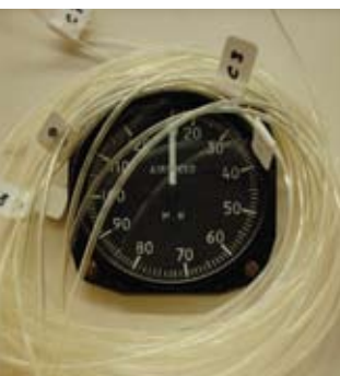
SMALL PLASTIC TUBES MEASURE WIND PRESSURE, WHICH DETERMINES LOADS ON BUILDINGS.
