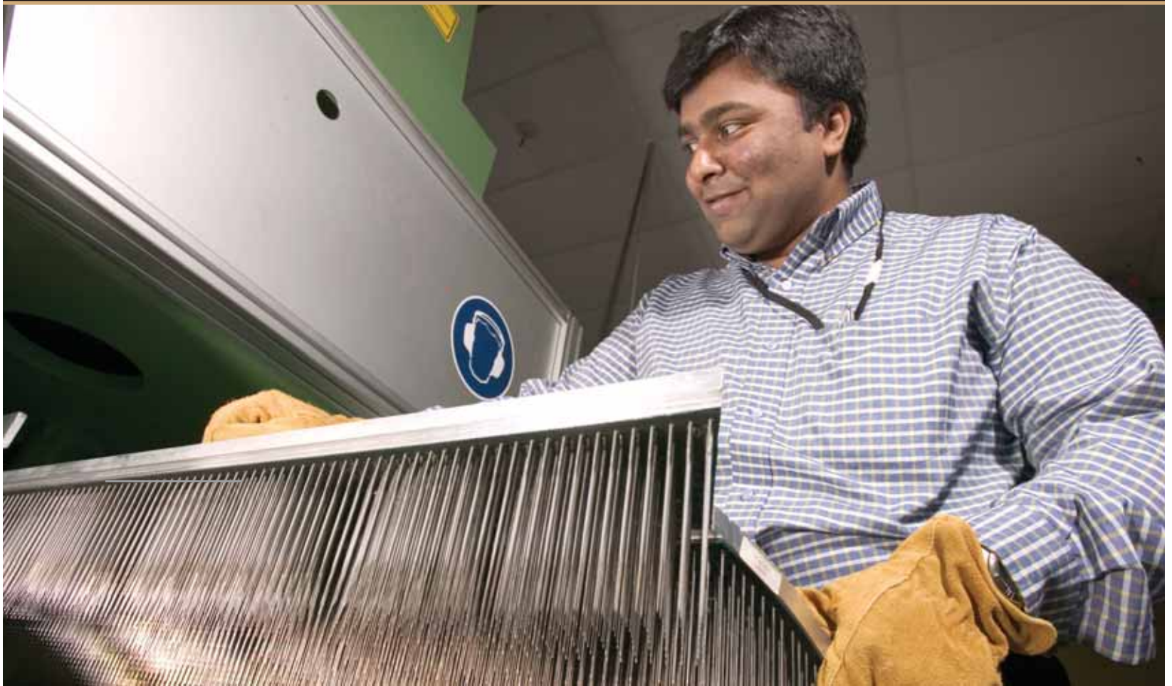
Research staff member Senthil Chinnasami installs a needle-board into TIEHH's needlepunch loom.
