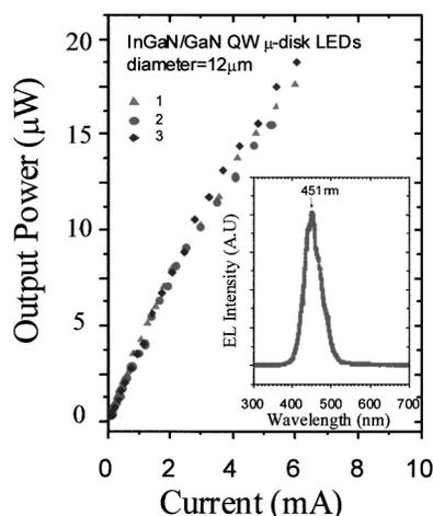
FIG. 2.  $L$ - $I$  characteristics (output power vs forward current) for three individual  $\mu$ -disk LEDs within the microdisplay of Fig. 1(b) measured through the sapphire substrate on unpackaged chips. The inset is the electroluminescence (EL) spectrum of a blue  $\mu$ -disk LED.
