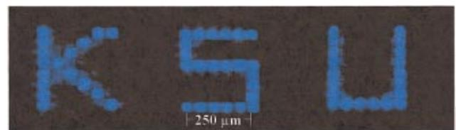
FIG. 3. (Color) Optical microscope images (top view) of the III-nitride blue microdisplay of Fig. 1(b) in action, displaying letters "KSU" demonstrating the operation of a semiconductor microdisplay.
