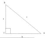
3. A surveyor needs to find the distance across a straight river. Markers are set up at points A and B on opposite sides of the river (see diagram), and at point C that is 260 feet from B, the angle at C is measured and found to be  $37^{\circ}$ . The angle at B is a right angle. Find the distance from A to B.
