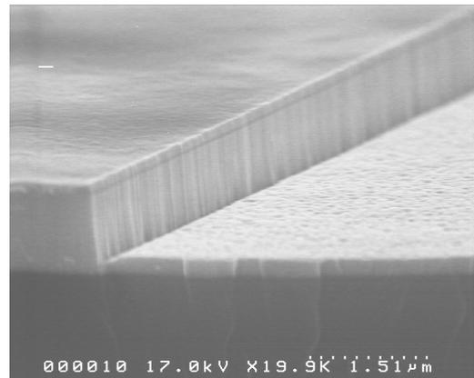
Fig. 5 SEM showing typical anisotropy of etched devices.
