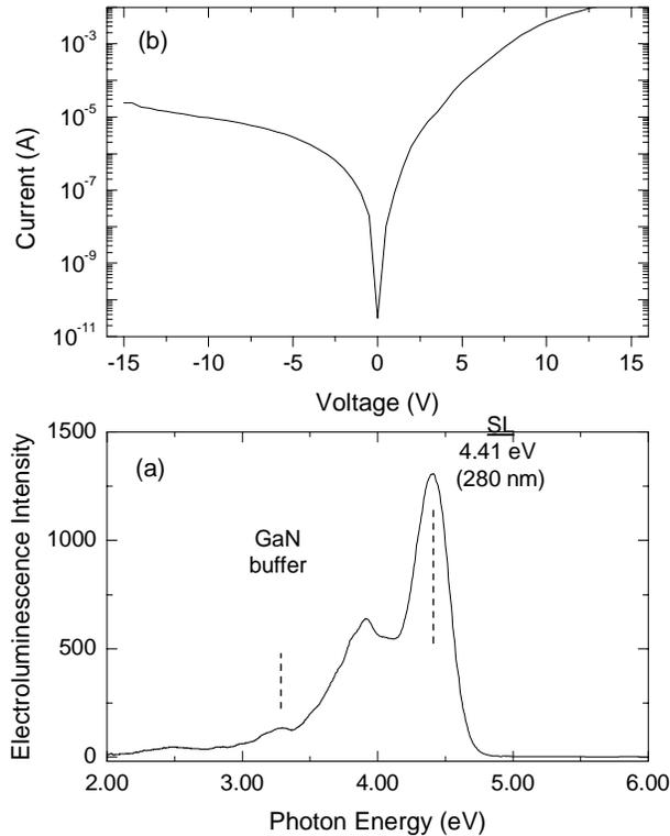
Fig. 6 (a) Electroluminescence spectrum of LED showing 4.41 eV emission. (b) Room temperature I-V characteristics.
