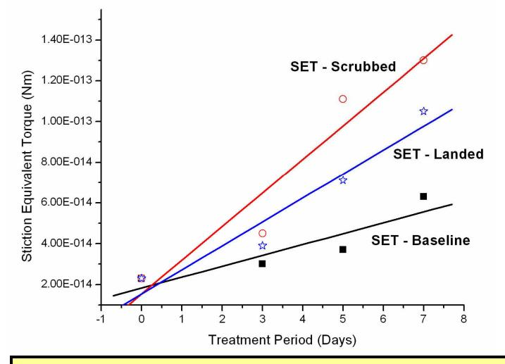
Increase in the stiction equivalent torque is highest in the case of the Scrubbed device for the treatment period
