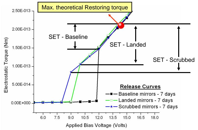
Stiction Equivalent torque translates Release Voltages into easily comparable torque values
