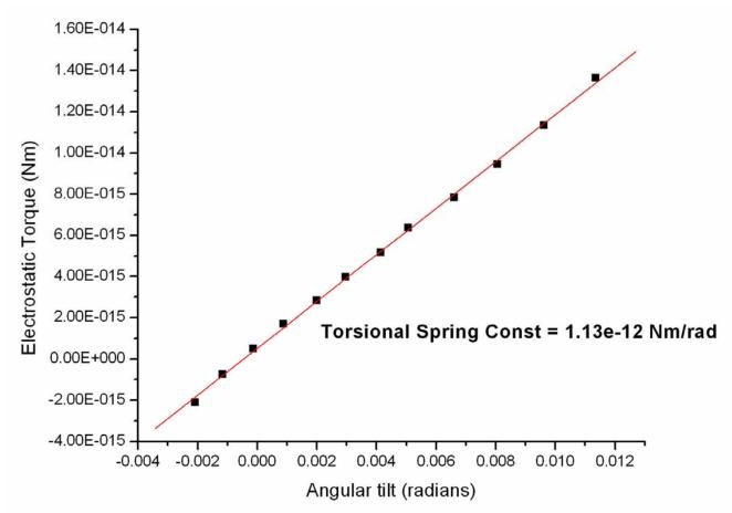
Maximum Restoring Torque = Spring Constant \* Maximum angular deflection
