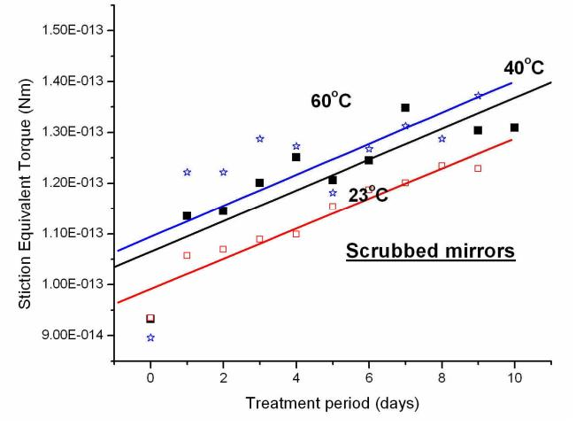
Change in the Stiction Equivalent torque with period of treatment is similar for the Scrubbed and Landed devices
