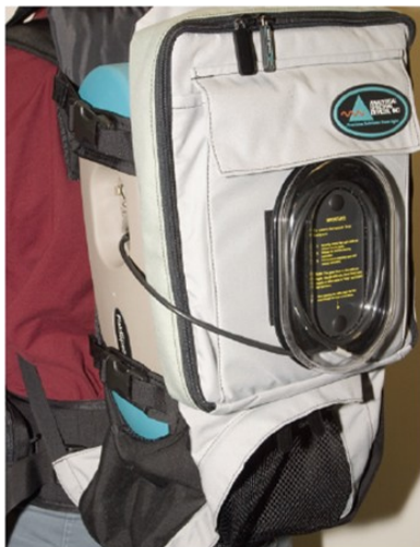
(Above) – The new spectrometer can be put into a backpack for field measurement, and is very portable.
