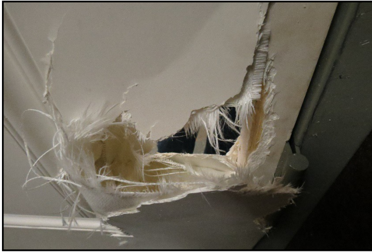
Figure 21: Perforation at center hinge.
