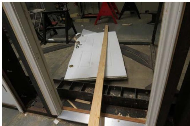
Figure 20: Series 1 door knocked from frame and twisted by first impact.
