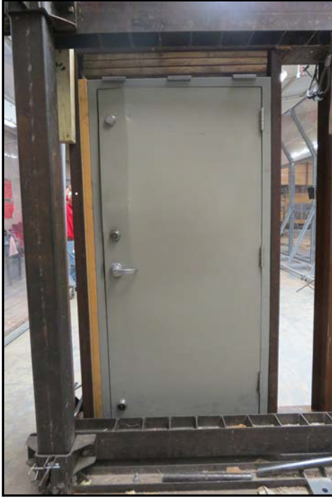
Figure 46: Vertical stiffener imprint after 2 Impacts.
