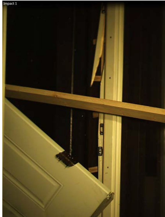
Figure 19: Series 1 door twisted 180 degrees by impact.
