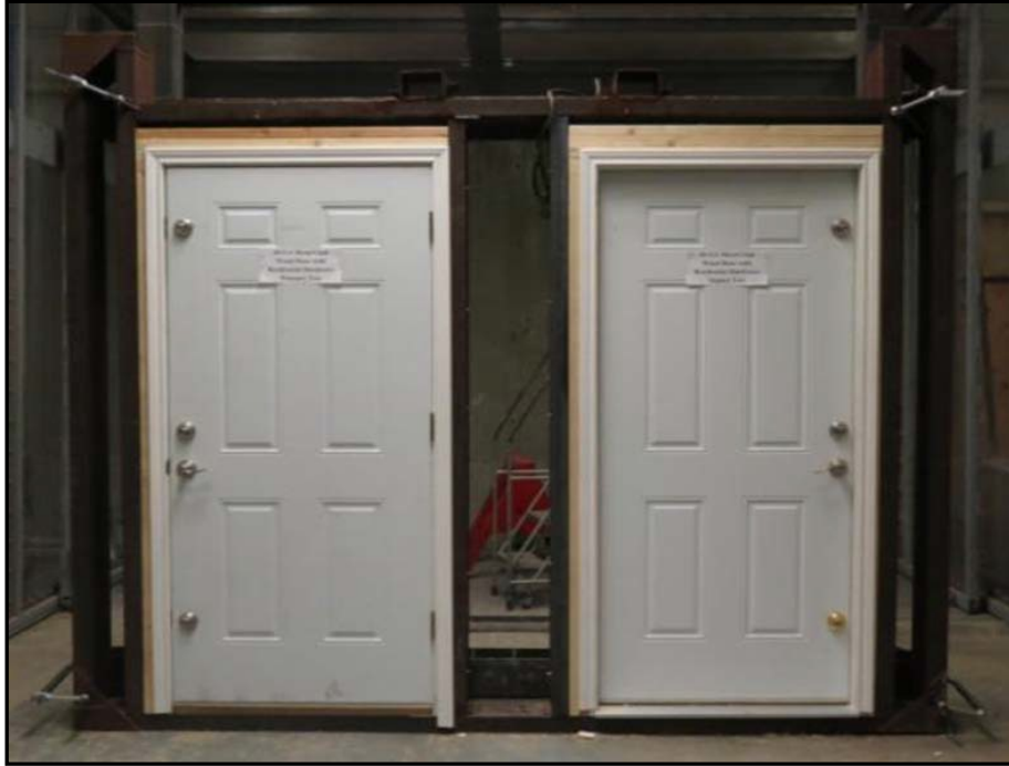
Figure 9: Series 1 Out-swing Pressure Door Left and In-swing Impact Door Right.
