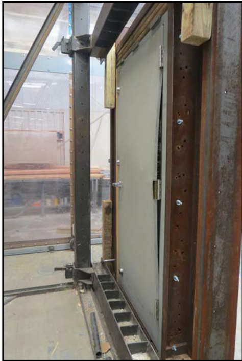
Figure 48: Sheet separation produced by Impact 3.
