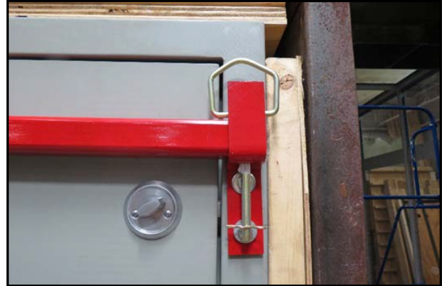
Figure 39: Safety pins installed on all shear pins.
