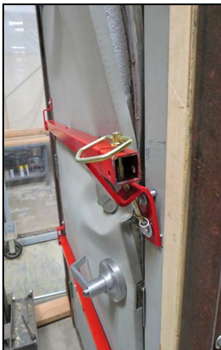
Figure 37: Impact 2 on Crossbar w/ shear & safety pin
