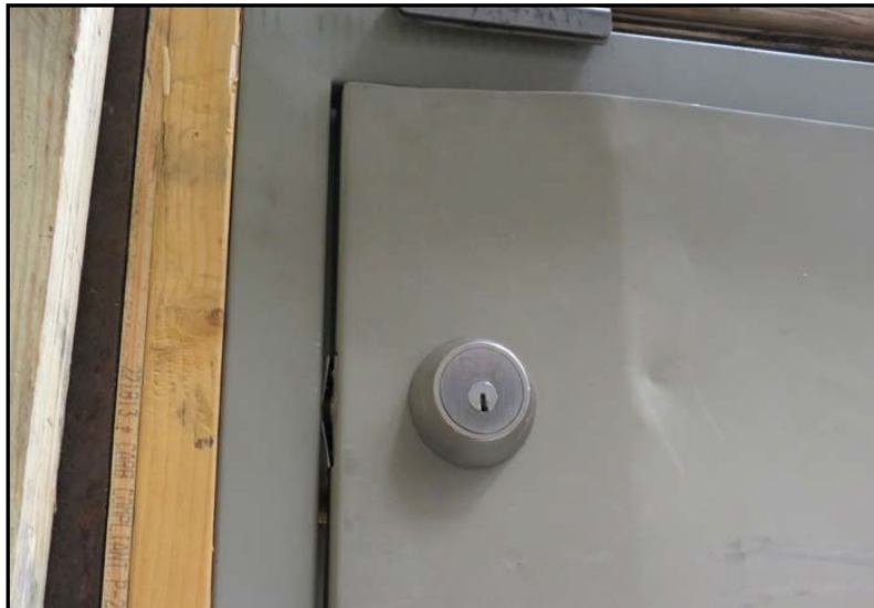
Figure 45: Backside damage after Impact 1.
