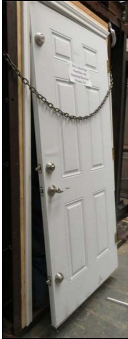
Figure 12: Series 3 Pressure Failure.
