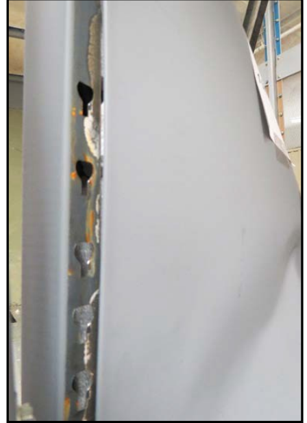
Figure 28: Series 3 door bellied and delaminated.
