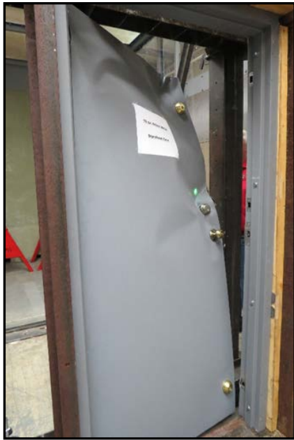
Figure 31: Bottom two deadbolts withdrawn.
