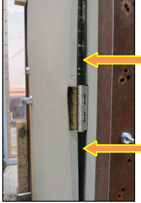
Figure 49: Delamination of back face sheet.
