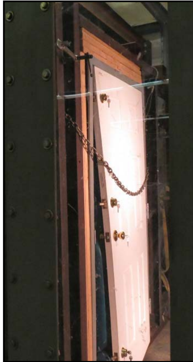
Figure 14: Series 2 Pressure Failure.
