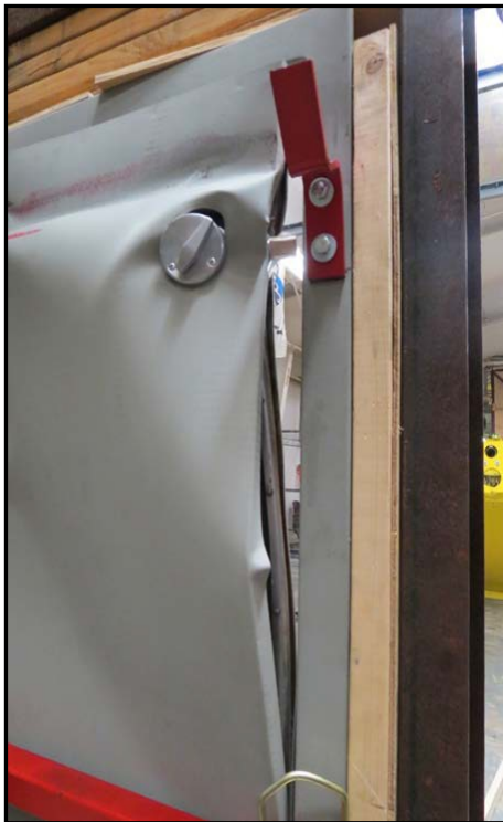
Figure 35: Cross bar removed by Impact 1
