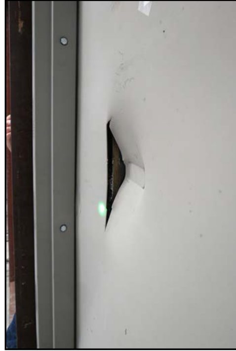
Figure 47: Sheet tear by Impact 3.
