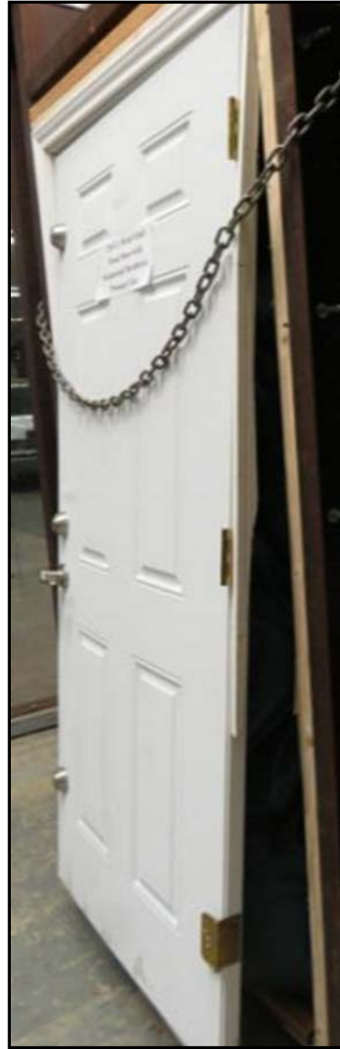
Figure 13: Series 3 Hinge Jamb Split.
