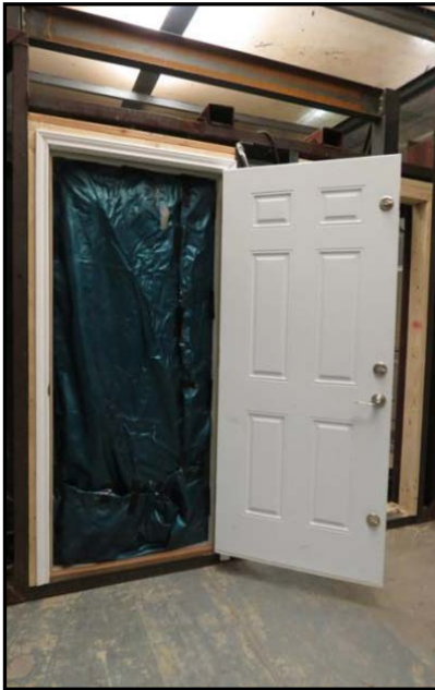
Figure 10: Bladder Installed for Pressure Test.
