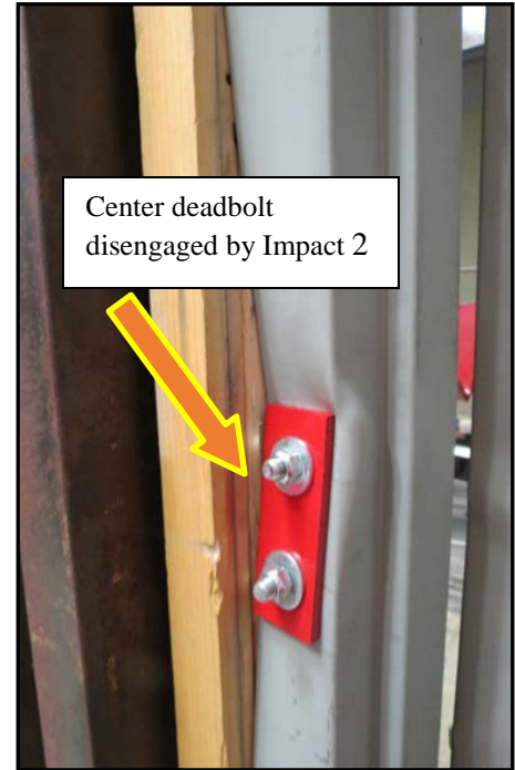
Figure 42: Frame crushed by hanger plate
