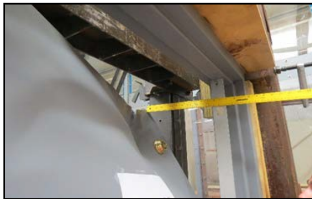
Figure 30: 12-in. door corner deflection.
