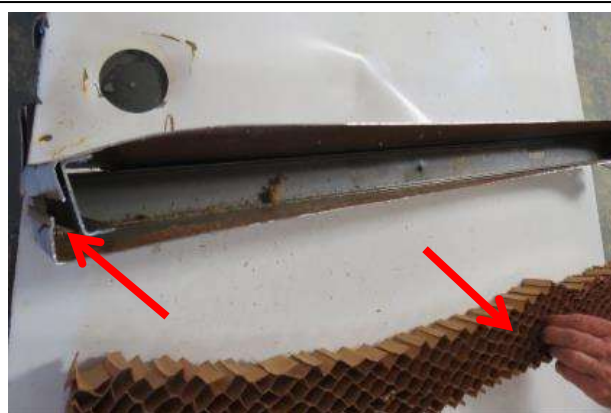
16 ga. Edge Channels and honeycomb core
