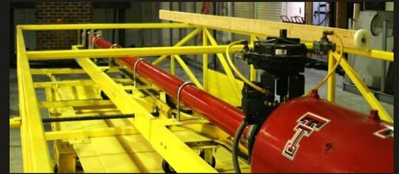
The heart of the DIF is a pneumatic cannon that plays an important role in researching effective tornado shelters for use in homes and other structures. The cannon is used to develop standards for safe above ground shelters, and continues to be in demand for testing new shelter materials and constructions.
