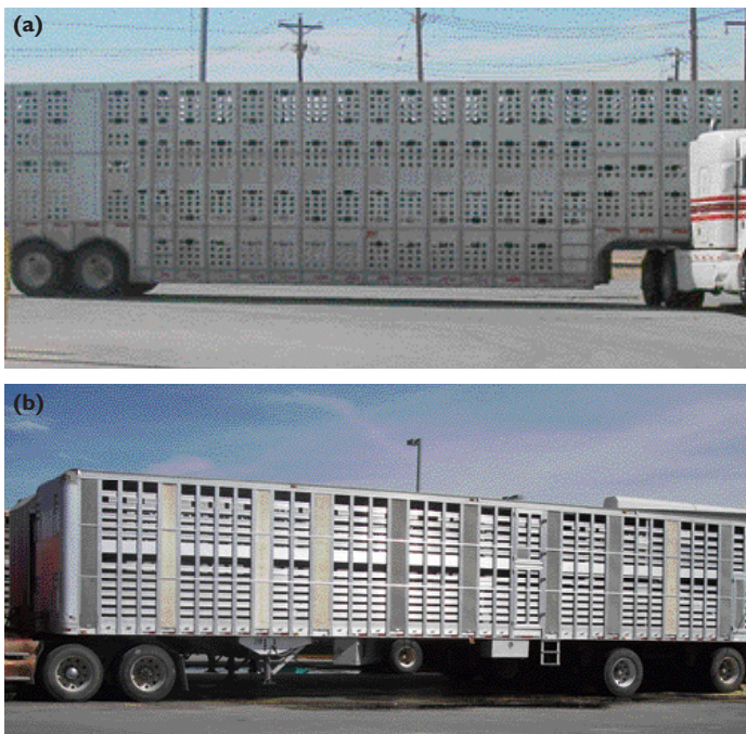
FIG 1: Examples of (a) a pot-belly trailer and (b) a straight-deck trailer used to carry pigs
