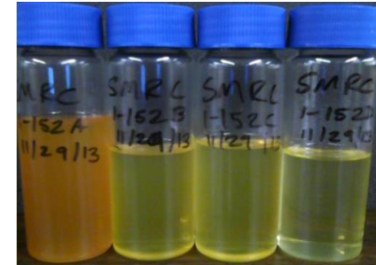
Nanosilicon suspensions in RP-2 from 1.0-0.1 wt% (left to right) after 24 hours
