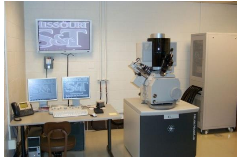
Focused Ion Beam (FIB) Inspection system
