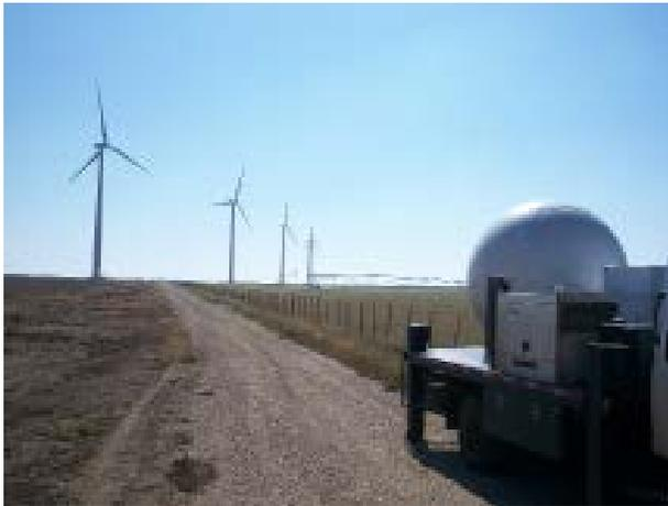
National Wind Institute researchers developed a new radar system capable of measuring wind flow within wind energy plants.
