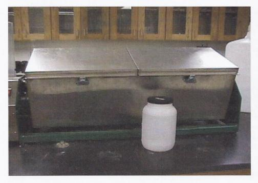
Figure 2: Extraction Vessel and Tumbler
