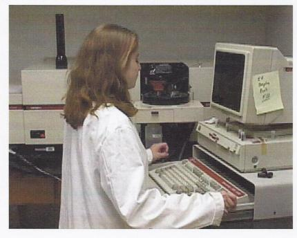
Figure 1. Graphite Furnace Atomic Absorption Spectrometer
