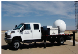
One of the two TTU Ka-band mobile Doppler pulse compression systems utilized in WISE research.
