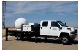
One of the two TTU Ka-band mobile Doppler pulse compression systems.
