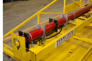
The debris impact cannon at NWI.
