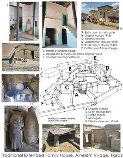
Fig. 8: This traditional well maintained extended family hidmo compound in Ainelem Village will soon have parts of buildings E & D demolished to gain a 1.5m wide strip of space for road widening.
