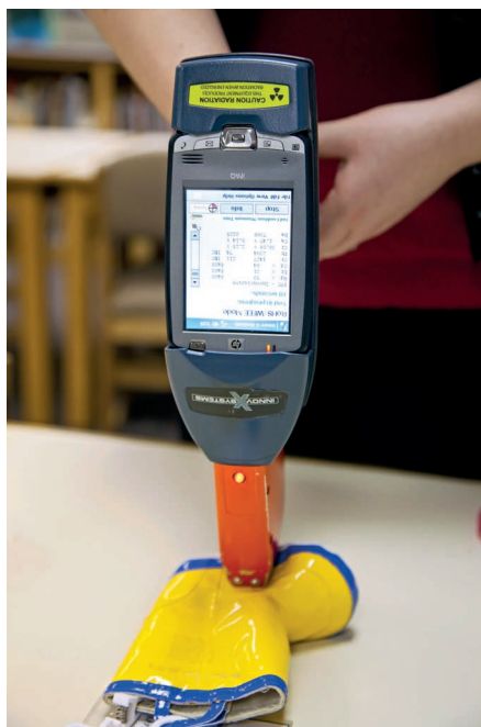
A hand-held X-ray fluorescence spectrometer is used to test for toxic chemicals in a child's boot.
