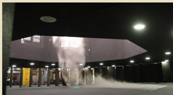
The new VorTech is simulating a tornado
