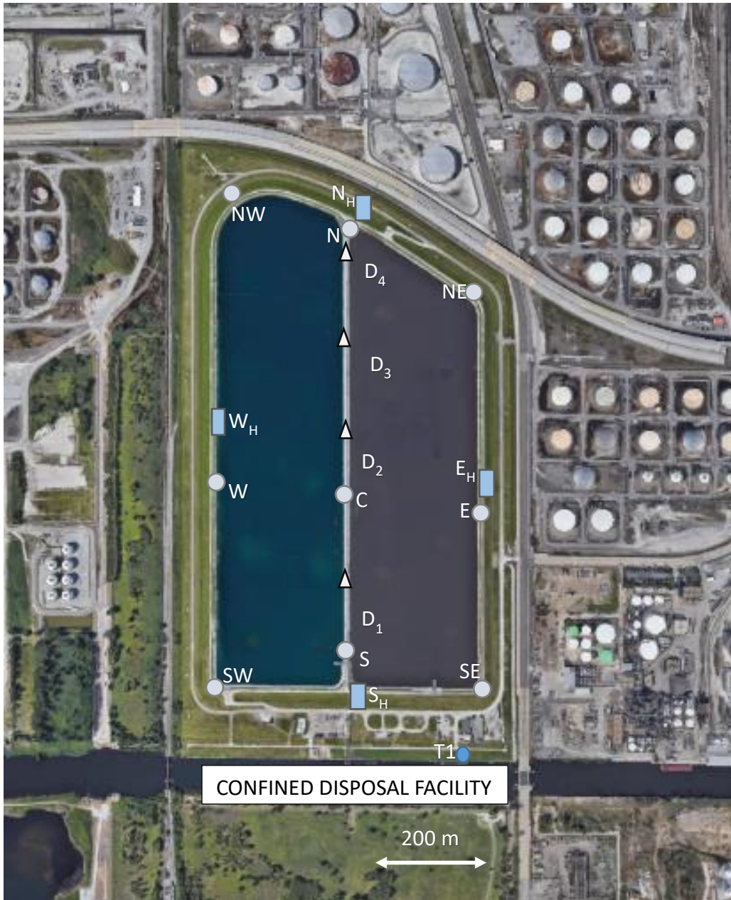
Figure 5.1. Overhead photograph of CDF and adjacent industrial facilities. POM sampling locations are denoted by circles, HVAS sampling locations by rectangles and dredged material discharge locations by D1 through D4.
