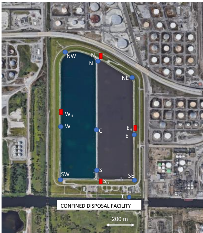
Figure 4.1. Overhead picture of the CDF and the surrounding industrial areas showing the 10 locations for PAS with 9 location around the perimeter of the CDF and a location AD near the administration office, and 4 locations for HVAS at the four cardinal directions namely S_H , E_H , N_H and W_H .
