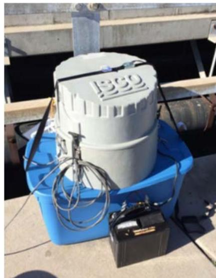
**Figure 4-3:** ISCO autosampler.
