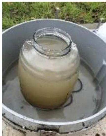
**Figure 4-4:** Stormwater sample collected in a 10 L carboy.
