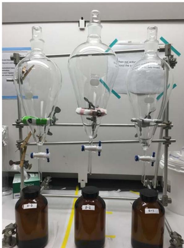
**Figure 4-9:** 2-L separatory funnel setup.
