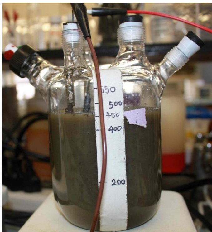
Figure 3.5 The reactor for electrode enhanced biodegradation experiment
