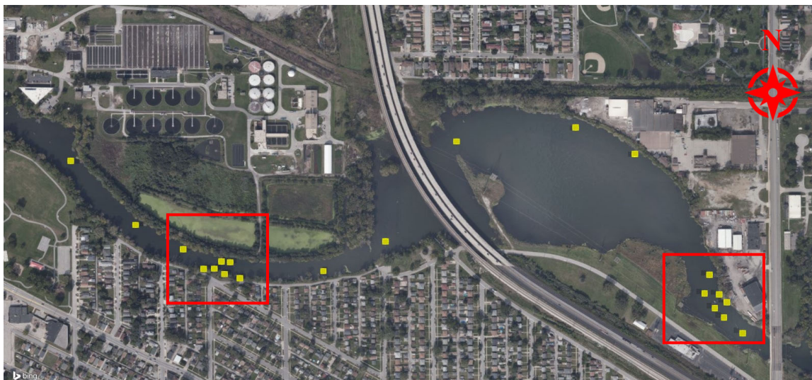
Figure 6-1 SPME PDMS long-term monitoring stations within the West Branch of the Grand Calumet River. Area 1 is in reference to the east sampling section and Area 2 represents the west sampling stations
