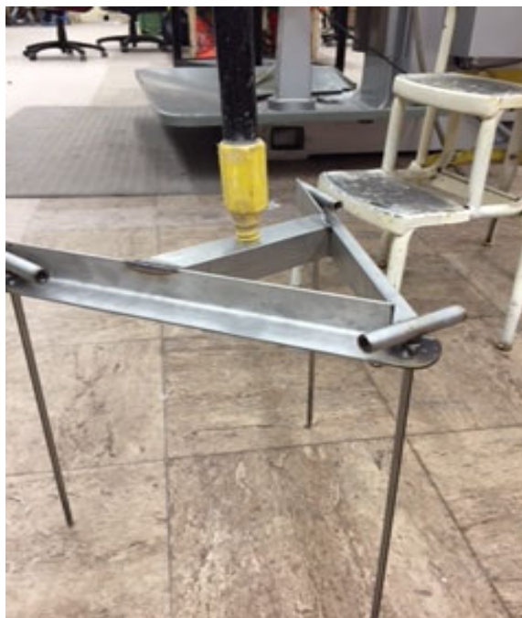
Figure 7-4 Tripod sample holder for in-situ passive sampling. Each SPME sampler contains two 30-cm PDMS fibers. The yellow and black deployment rod is fastened onto the top of the tripod for ease of deployment in deeper surface waters and is easily removed
