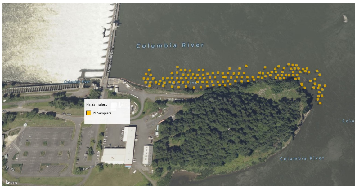
Figure 4-3 LDPE sampling stations along the Bradford Island shoreline. A total of 163 LDPE samplers were deployed
