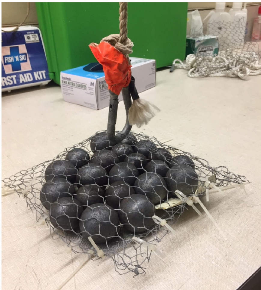
Figure 4-1 LDPE sampling apparatus for Bradford Island. The LDPE samplers (10 cm x 10 cm coupon) is placed underneath the steel balls in a stainless-steel wired mesh and lowered down to the sediment water-interface
