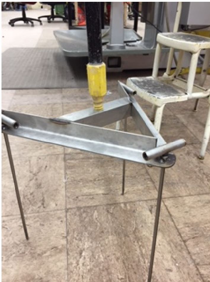
Figure 3-6. Passive sampling tripod employed at each field location
