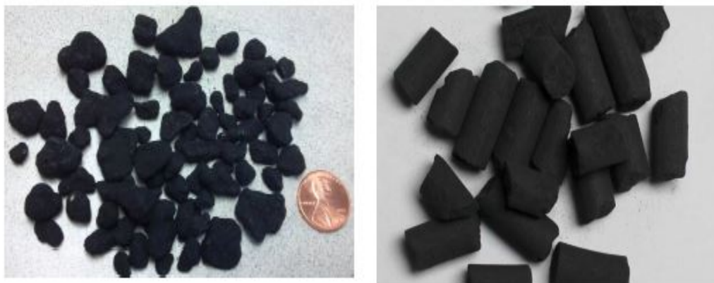
Figure 4-4. Two type of amendment materials used at Hunter's Point Navy Shipyard: AquaGate+PAC (left) and sedimite (right)
