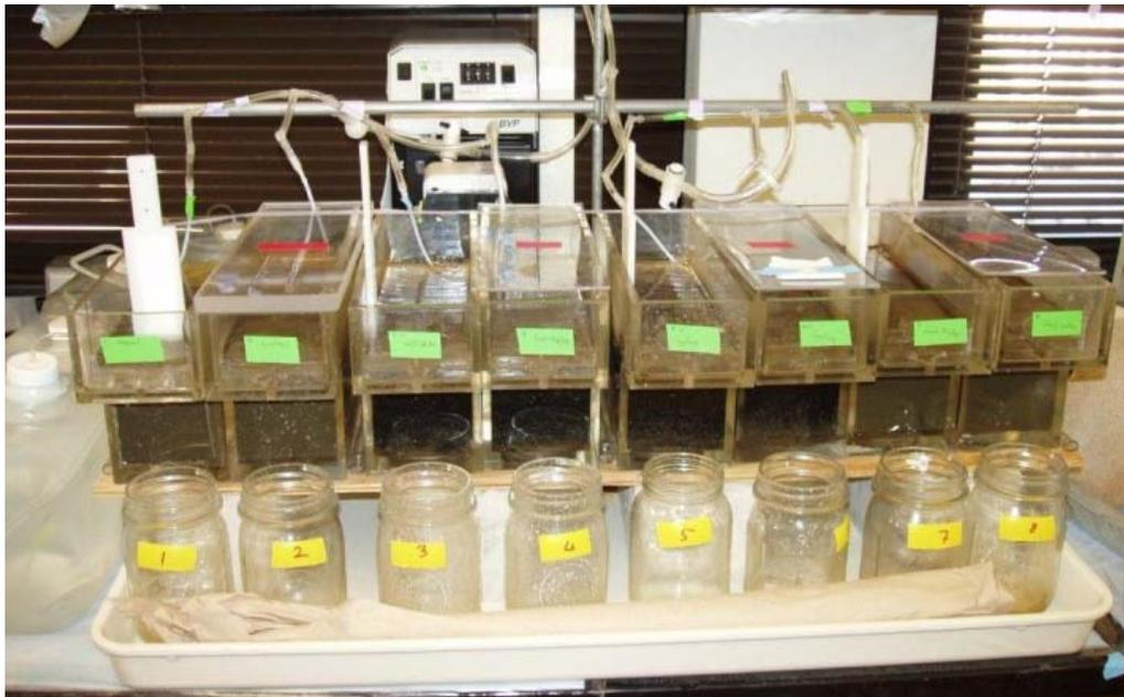
Figure B.2 Schematics and experimental setup of microcosms
