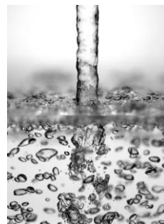
A plunging water jet entrains irregularly shaped air bubbles beneath the surface
