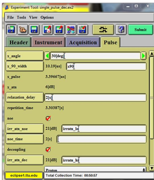
**Total Collection Time:** shows approximate time necessary for this measurement with current acquisition parameters. Always check that value before starting  $^{13}\text{C}$  acquisition since this can be rather long experiment (many scans and long relaxation delay).
