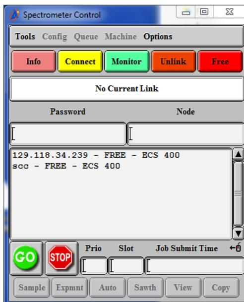
Eclipse 1 displays: **eclipse1 – FREE – ECS 400** while Eclipse 2 displays: **scc – FREE – ECS 400**. Select the spectrometer by clicking that line and then click the **Connect** button. The spectrometer marked as **FREE** is available for connection. The spectrometer marked **OWNED** or **ACTIVE** is currently being used and only the Monitor mode is available. If the console is available
