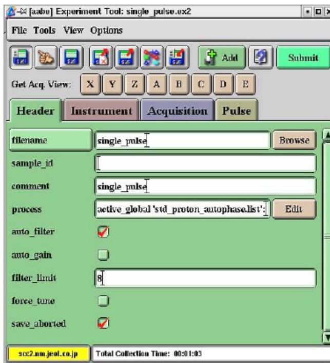
The Experiment Tool window consists of the four sections (tabs): Header, Instrument, Acquisition, and Pulse. Acquisition parameters can be displayed by clicking on these tabs.
