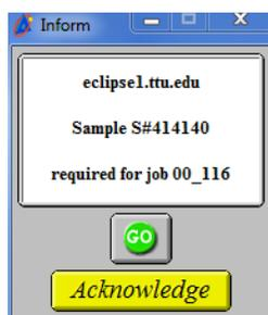
The experiment is entered into the spectrometer control queue (see below). The spectrometer executes measurement on a first-in, first-out basis. Commands for starting acquisition can be issued repeatedly, even if another measurement is being performed. After one experiment finishes, the data is auto-saved and the next experiment will be started, using the stored acquisition parameters.
