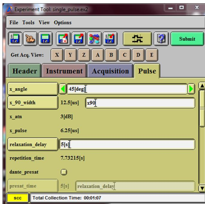
**Total Collection Time:** shows approximate time necessary for this measurement with current acquisition parameters
