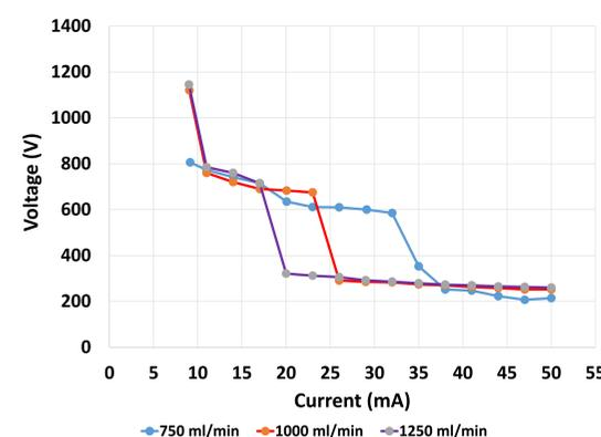
Figure 4. Characteristic current-voltage curve for FAPA.
