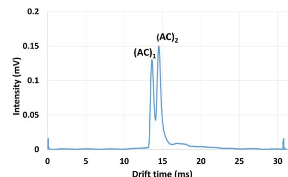
Figure 7. Ion mobility spectrum of monomer and dimer of acetone at 13.8 and 14.3 ms, respectively ( $\text{AC}_1$  and  $\text{AC}_2$ ).
