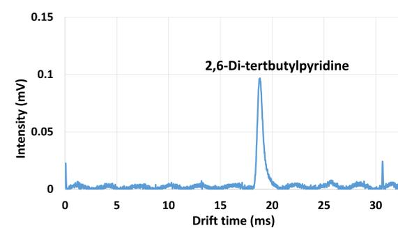
Figure 6. Ion mobility spectrum of 2,6-Di-tertbutylpyridine at 19.1ms
