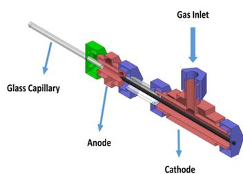
Figure 2. Section view of FAPA.
