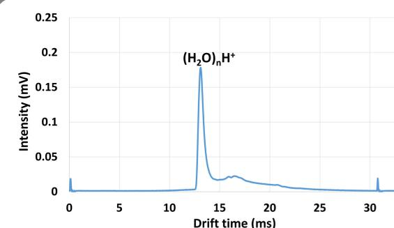
Figure 5. Ion mobility spectrum of reactant ions formed in FAPA source at 12.9ms (no sample).
