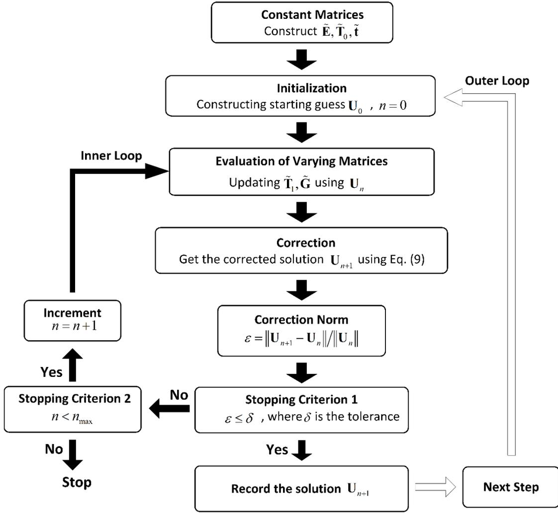
Figure 1 The flow chart of OFAPI method for solving nonlinear differential equations
