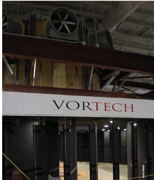
The VorTECH simulator uses large fans to pull air up, while vanes surround the simulator to create rotation.
