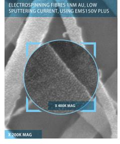
Ultra-fine grain size coating and high density allows for imaging a fibre's discrete morphology - like steps, tears or inclusions, even for fibres as small as 10nm diameter.
