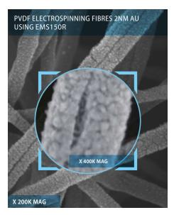
Dense coating allows for good imaging contrast, although further investigation of a single fibre morphology is difficult. The coating tends to glue together fibres that are close together, making them look like one.
