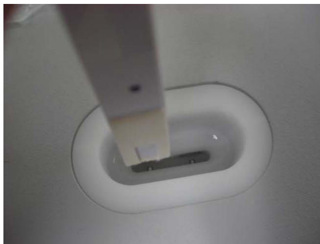
Orientation of swab to cell for cleaning
