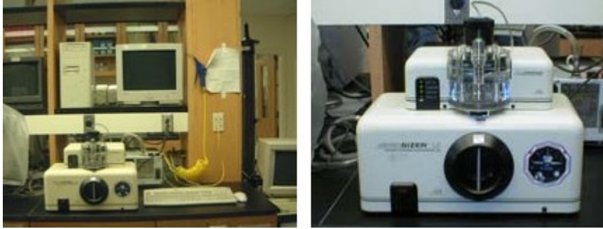
Figure 1: The API Aerosizer particle size analyzer consists of an API Aerosizer LD sensor unit, an API Aero-Disperser dry powder dispersing system fitted to the API Aerosizer LD, a controller, and a vacuum pump.
