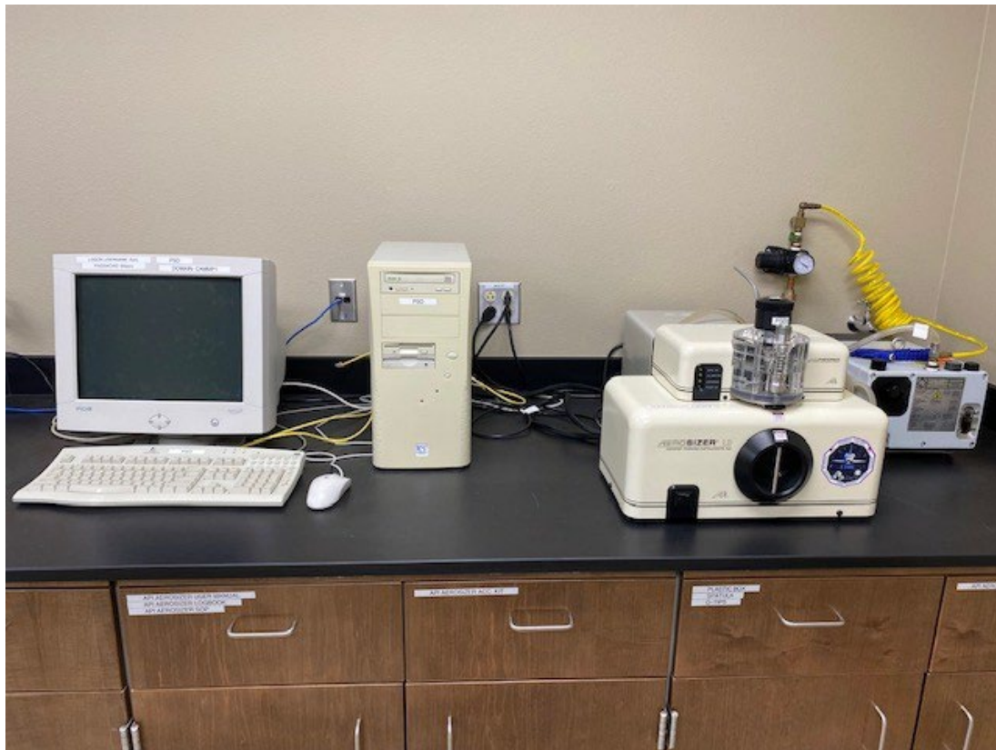
Figure 1. The API Aerosizer particle size analyzer consists of an API Aerosizer LD sensor unit, an API Aero-Disperser dry powder dispersing system fitted to the API Aerosizer LD, a controller, and a vacuum pump.
