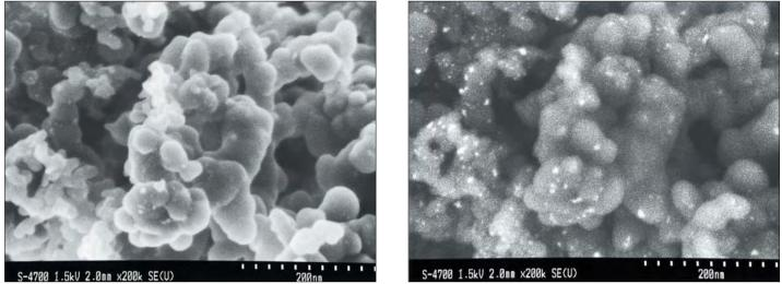
The SE image shows topographic details of the specimen surface at high resolution. The SE + BSE image shows specimen compositions reflecting atomic number contrast.
