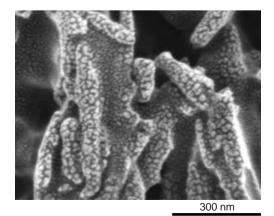
High resolution micrograph of gold coated magnetic tape, recorded at 0.5 kV and WD of 2.5 mm, courtesy of Nissei Sangyo America, U. S. A.
