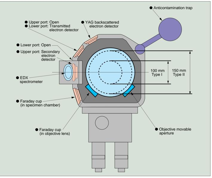
The S-4700 has a large and versatile specimen chamber as illustrated above. Depending on the specimens and applications, SEM users can choose either a large or small specimen stage, as shown on the right. Various accessories, such as a backscattered electron detector, cryogenic system, or energy dispersive X-ray spectrometer, can be accommodated with the S-4700 chamber. These accessories extend the use of the S-4700, for a wide range of analysis possibilities.
