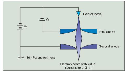
The table below is a comparison of various SEM electron sources. It is obvious that the cold field emission suppplies an optimum set of operating parameters and is the most promising electron source for ultra-high resolution microscopy, specifically in terms of source brightness, source size, emission current, energy spread and service life.
