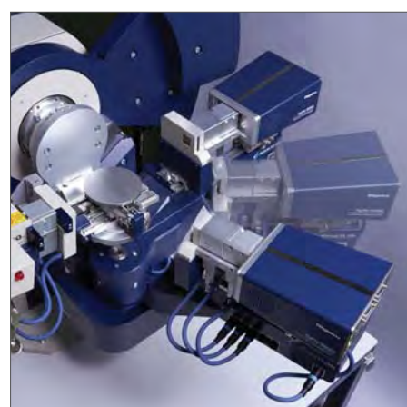
Fully compatible with 5-axis goniometer design
