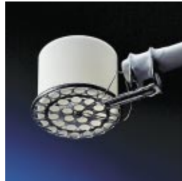
Large sample holder with 900 µl aluminum oxide crucible.
