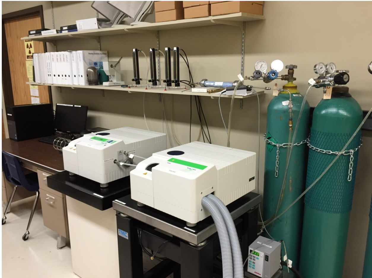
Figure 1: Systems for Thermogravimetric Analysis and a Differential Scanning Calorimetry.
