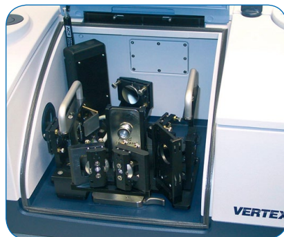
The large sample compartment accommodates virtually any FT-IR sampling accessory.
