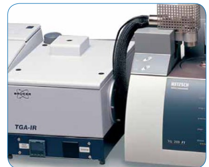
Many external accessories, such as the TGA module, can be coupled to the VERTEX 70.
